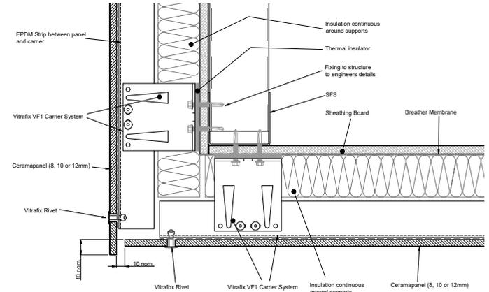
**VITRADUAL® CASSETTE FIX SOFFIT JUNCTION DETAIL**
