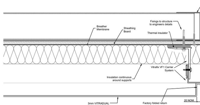
**CERMAPANEL® RIVET FIX SOFFIT JUNCTION DETAIL**
