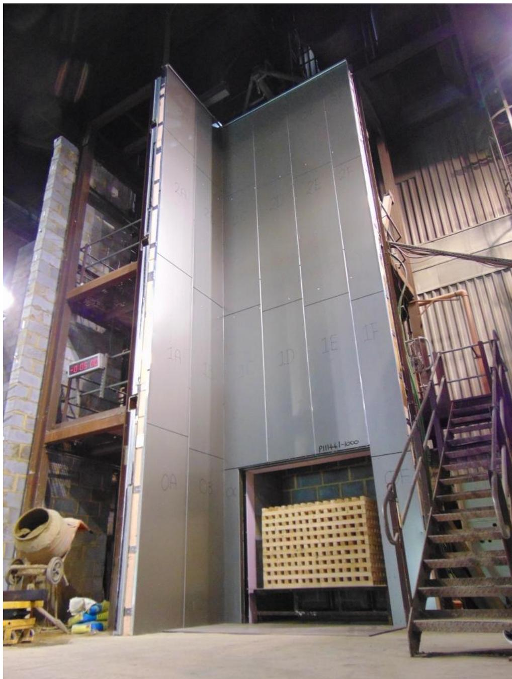
Figure 1. Full-height photograph of cladding system prior to test.
