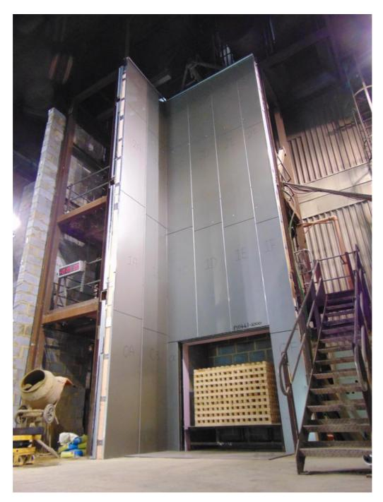
Figure 1. Full-height photograph of cladding system prior to test.
