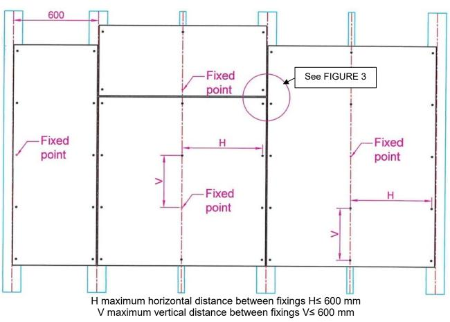
FIGURE 2.1: FIXED POINT ON FIBRE-CEMENT FLAT SHEETS
